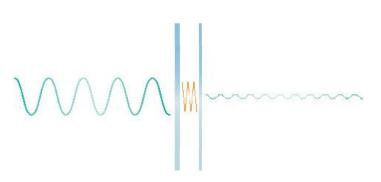
Figure 5 Sound waves as they propagate through laminated glass constructed with an acoustic interlayer. Source: Australian Fenestration Training Institute.
