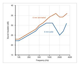
Figure 4 Acoustic Performance Comparison: Laminated
