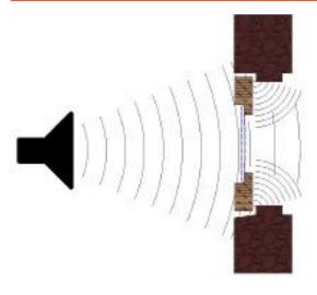
**Figure 2** Sound Propagation Through a Window
