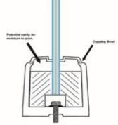
Note : Balustrade channel designs with a top cap or bead may create a potential internal cavity for water to pool. Also, where dry glazed systems are used, consideration must still be given to ensure that any water which enters the channel is able to drain away.
